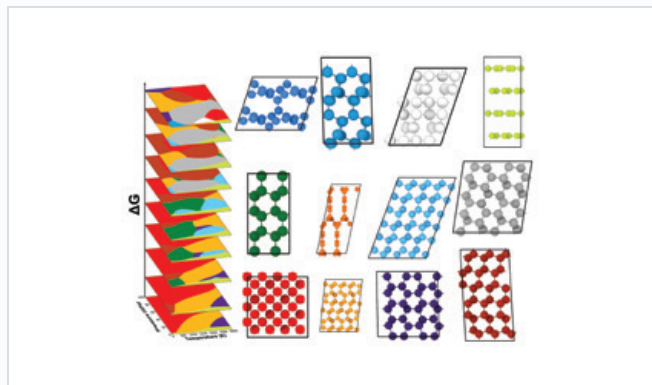
The final product of the machine learning algorithm: metastable phase diagrams for carbon. The colored regions indicate conditions at which carbon exists in certain metastable states (with similarly colored structures) that may yield useful material properties. Image: Argonne National Laboratory
