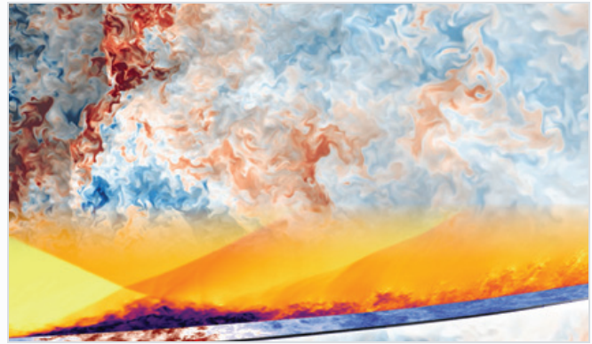
Different aspects of shock-turbulence interactions. Background: shock-induced mixing shadowed by the velocity marking the shock. Foreground: oblique shock impinging on a turbulent boundary layer over a flexible panel. Image: Ivan Bermejo-Moreno, University of Southern California
