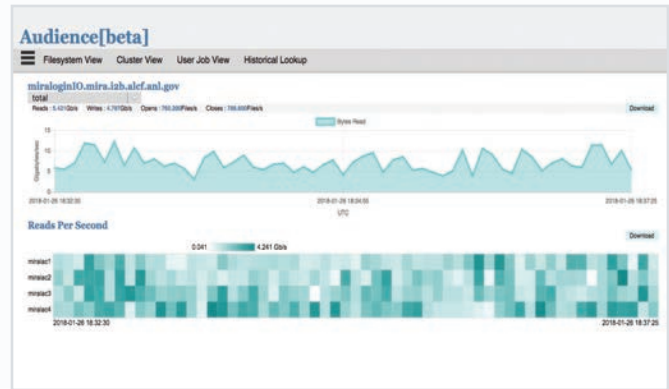
The Audience web application was developed to help staff members monitor file system traffic and performance on ALCF resources.
